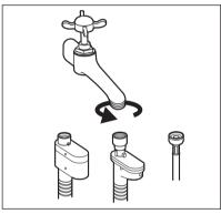
Connect the water inlet hose to the cold water tap with 3/4 thread.
